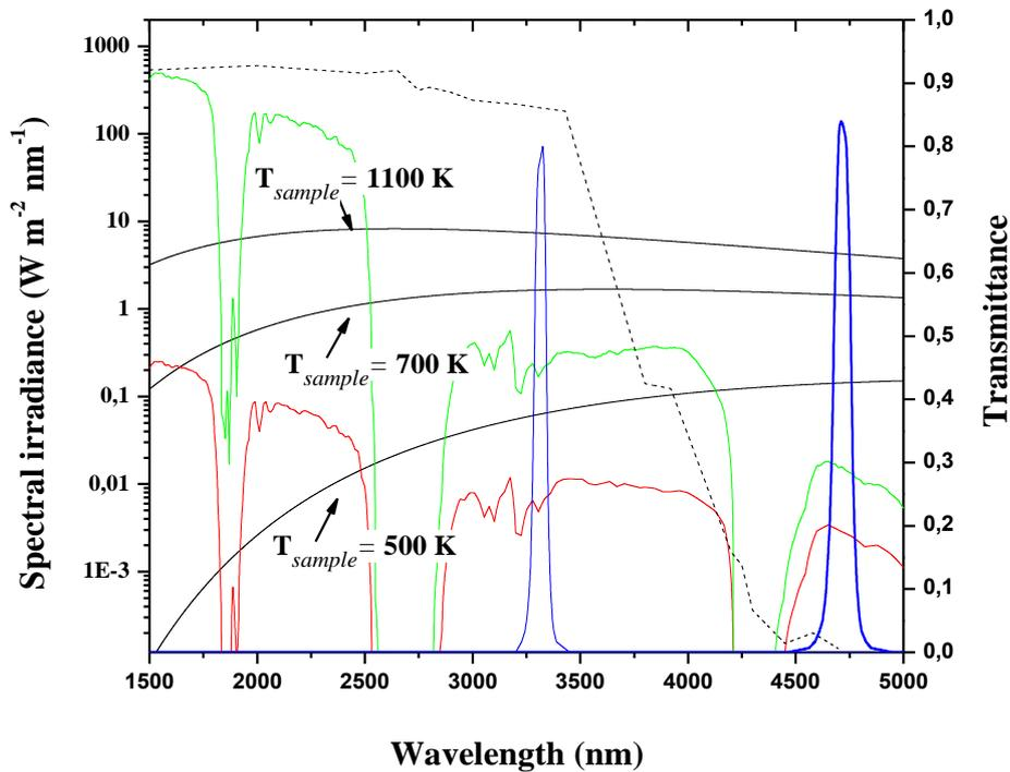
Figure 3.13. Solar spectrum based on a MODTRAN simulation (red line) and solar spectrum reflected by an opaque surface with a reflectance of 0.60 in the PSA solar furnace according to the concentration factor 3034X (green line), thermal irradiance at several temperatures of samples with an emittance of 0.40 (black lines), transmittances of band-pass filters at 3320 nm and 4720 nm (blue lines), and quartz transmittance (dotted line).
