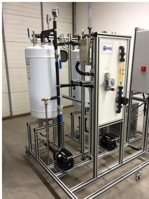
Figure 2.38. Laboratory unit for testing membranes on isobaric MD
