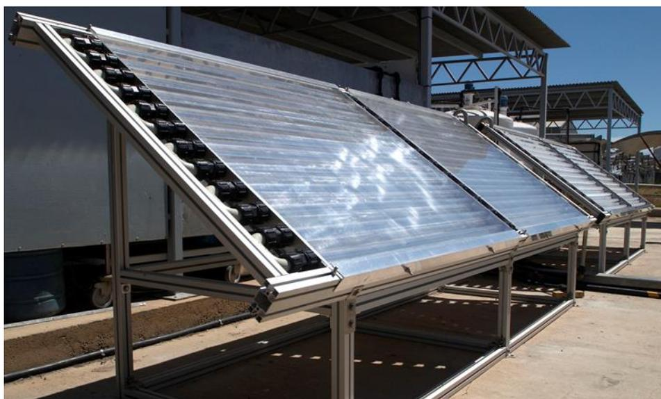
Figure 2.40. CPC photo-reactors (SOLEX prototype).
