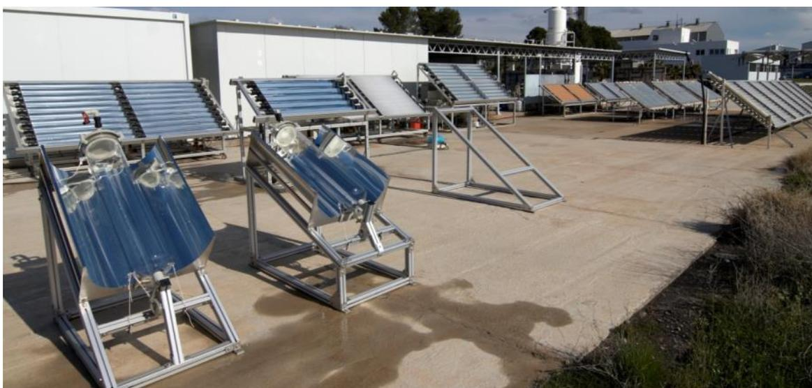
Figure 2.41. General view of several CPC reactors for decontamination and disinfection of water.
