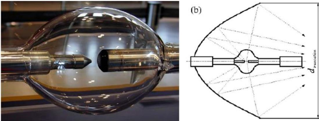
Figure 2.27. Xenon lamp used in the solar Simulator and configuration of the lamp and concentrator
