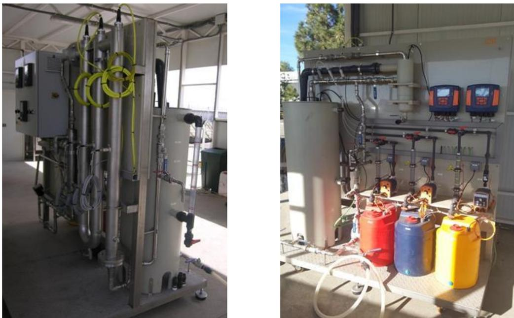
Figure 2.43. New UVC pilot plant. Three medium pressure UV lamps (254 nm) inserted in stainless steel frame (left view). Automatic dosing pumps for automatic control of pH and H<sub>2</sub>O<sub>2</sub> addition (right view).
