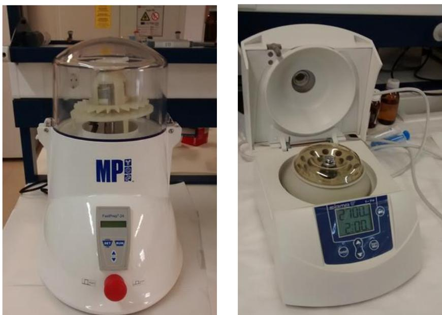
Figure 2.51. Left: 'Fast prep 24' biological homogenizer. Right: Micro-centrifuge.
