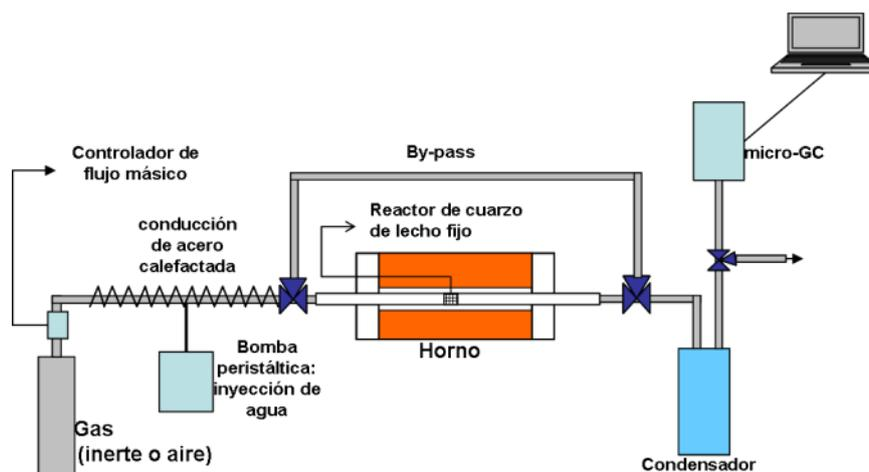
Figure 3.23. Diagram of bench test bed for the evaluation of the synthesized materials.
