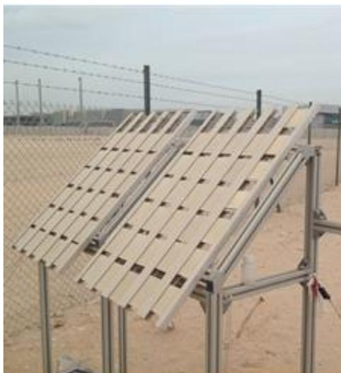
Figure 3.3. Aluminum reflector samples exposed in a desert area.
