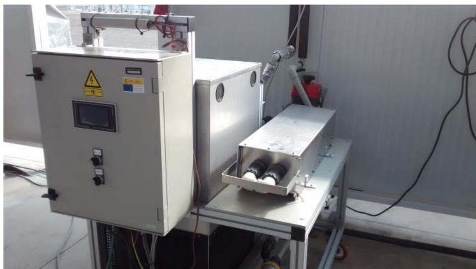
Figure 2.44. Module for temperature control in a CPC pilot plant for water disinfection.
