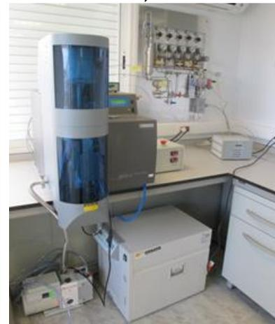
Figure 2.23. View of a) the Microscopy Room in the Materials Lab, b) Thermogravimetric balance inside of its Room at Materials Lab.
