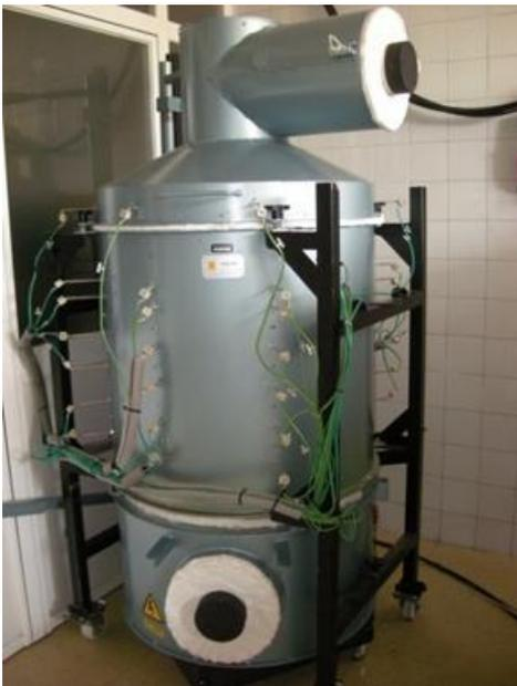
Figure 2.29. Front view of the lab-scale regenerative storage system in static arrangement.
