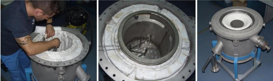
Figure 3.21. Oresol Reactor: Left: Insulation mounting. Center: Internals. Right: With window.
