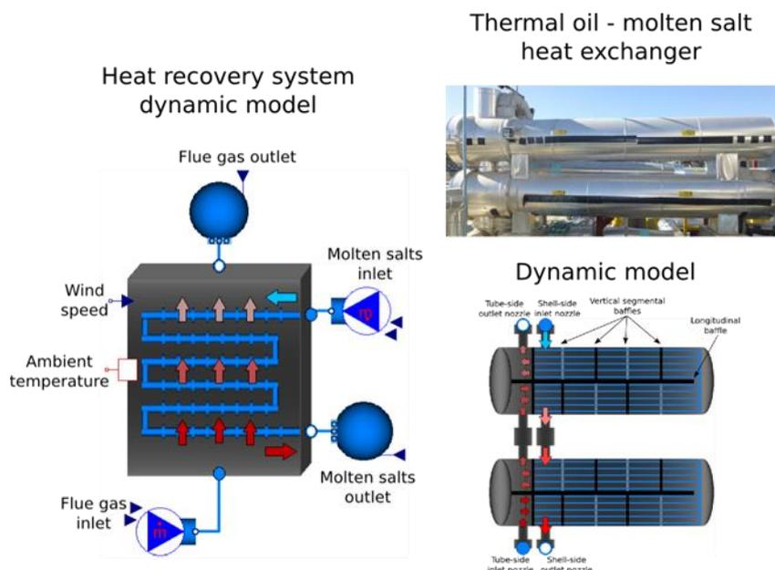
Figure 6.8. Heat recovery system and thermal oil - molten salt heat exchanger dynamic models.
