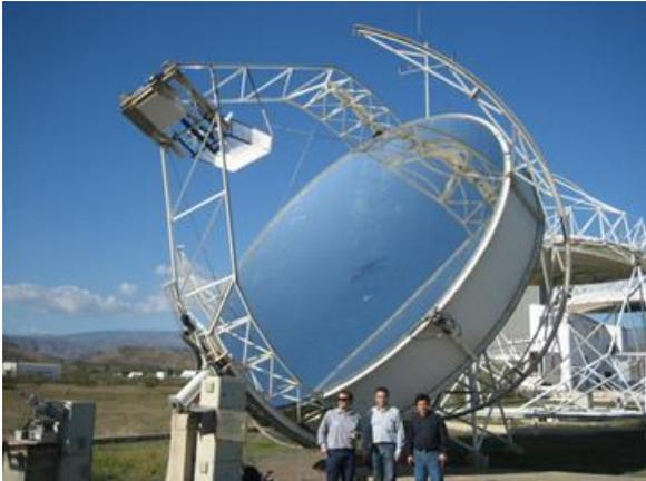
Figure 2.15. Parabolic-dish DISTAL-I used for accelerated materials ageing at PSA.
