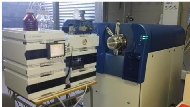
Figure 2.53. AB SCIEX TripleTOF 5600+ equipment.
