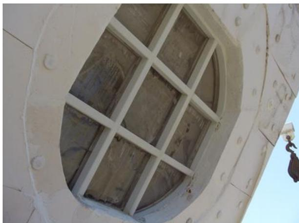
Figure 3.18. SYNPE500 reactor receiver window.
