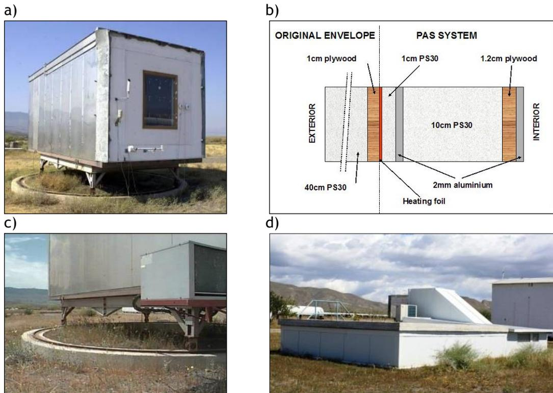
Figure 2.54. (a) CIEMAT's PASLINK test cell, (b) Schematic drawing of the PAS system, (c) Detail of the rotating device, (d) Exterior of the CETeB Test cell.
