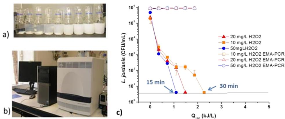
Figure 5.3. (a) Photocatalytic experiment using suspended TiO<sub>2</sub> (P25) at different concentrations. (b) Real time q-PCR (7500-Fast, Applied Biosystem) at PSA laboratory. (c) Inactivation of *L. jordanis* in distilled water using two enumeration techniques: real time q-PCR with EMA dye (empty symbols), and pour plate counting technique (solid symbols).
