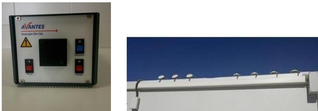
Figure 2.46. Spectral photometer AVANTES with double channel (left). View of all solar UV radiometers (inclined and horizontal setup) used in the Solar Water Treatment Unit (right).
