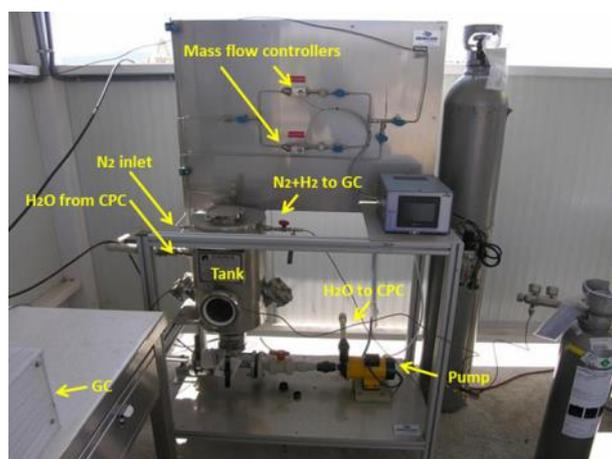
Figure 5.6. Solar pilot plant for photocatalytic generation of hydrogen.
