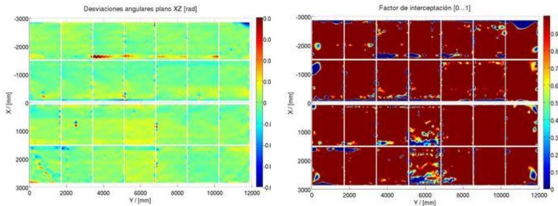
Figure 2.26. Angular deviations (left) and intercept factor (right) of a parabolic-trough collector module analysed by photogrammetry
