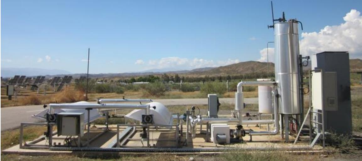
Figure 2.13. CAPSOL solar thermal test facility for small-size parabolic-trough collectors.
