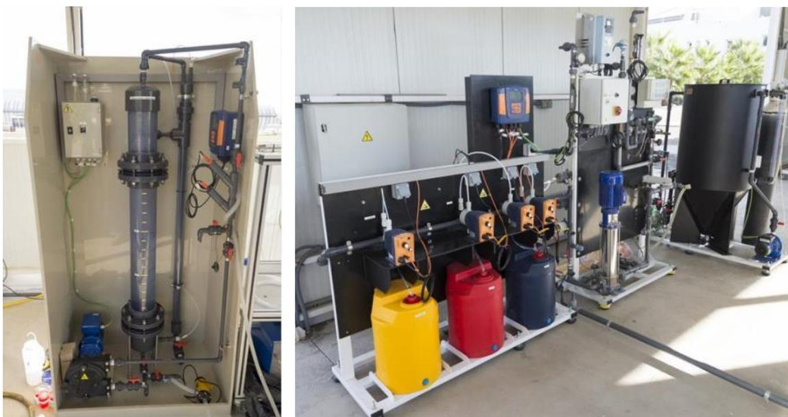
Figure 2.42. (left) New contact column reactor for ozonation system. (right) New configuration of the improved Nanofiltration membrane pilot plant.
