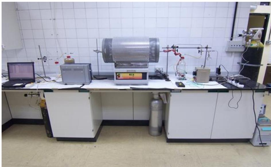
Figure 2.31. Solar Simulation Loop for evaluation of hydrogen production processes
