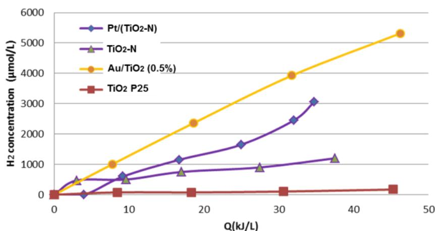
Figure 5.7. Hydrogen generated vs. accumulated solar UV energy (305-385 nm) for different photocatalysts at 0.2 g/L concentration. Reaction conditions: 25 L of 0.05 M formic acid aqueous solution at pH 3. Data corresponding to 5 hours of irradiation.
