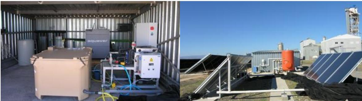
Figure 2.36. Internal (left) and external (right) views of the Membrane Distillation experimental test bed within the PSA low-temperature solar thermal desalination facility
