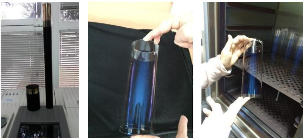
Figure 3.2. Selective absorber and borosilicate glass AR coating developed in CIEMAT/PSA
