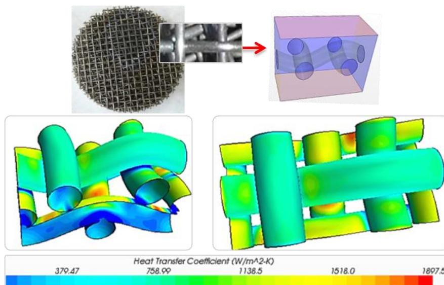
Figure 3.9. Absorber representative structure and model results
