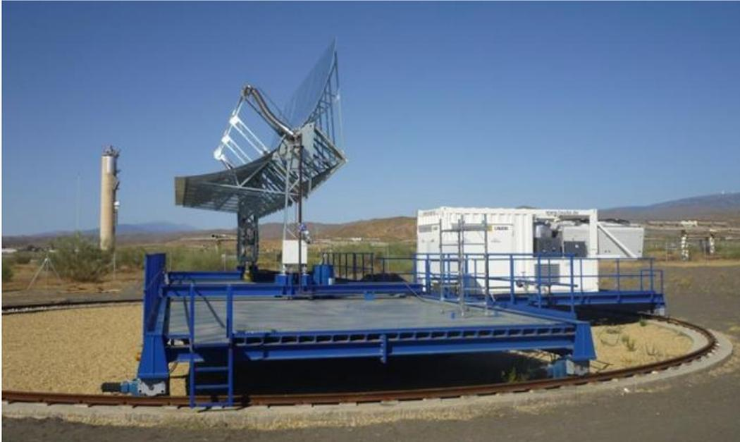
Figure 2.14. Side view of Kontas test bench and the heating cooling unit.
