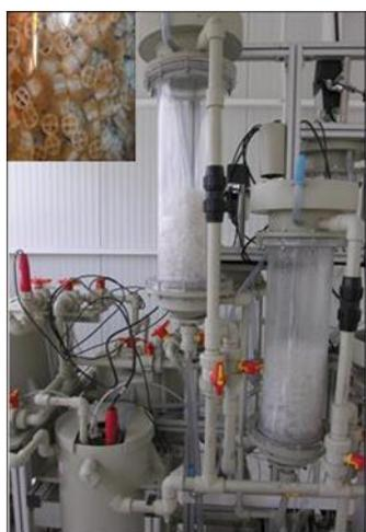
Figure 5.5. Biological post-treatment in an Immobilized Biomass Reactor at pilot plant scale of cork boiling wastewater partially oxidized by solar photo-Fenton process
