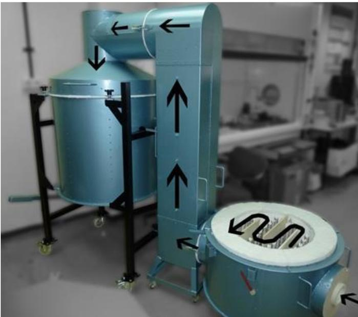
Figure 2.30 Front view of the lab-scale regenerative storage system in dynamic arrangement.
