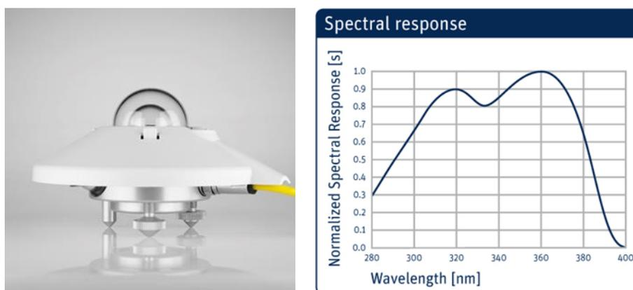
Figure 2.45. CUV-5 radiometer (left) and spectral response of CV-5 (right).
