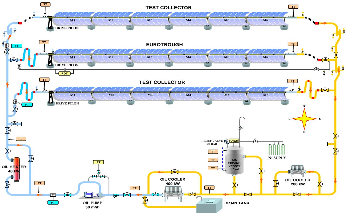
Figure 2.5. Diagram of the PSA “HTF test Loop”.
