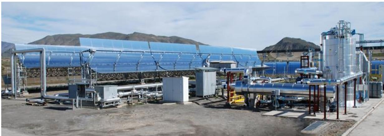
Figure 2.8. View of the pressurized gas test loop connected to a molten-salt thermal energy storage
