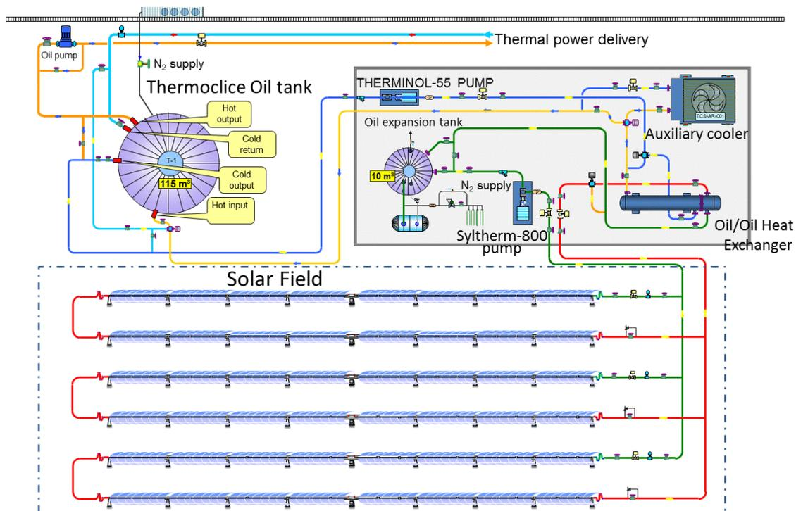
Figure 2.10. Diagram of the TCP-100 2.3-MWth parabolic-trough facility
