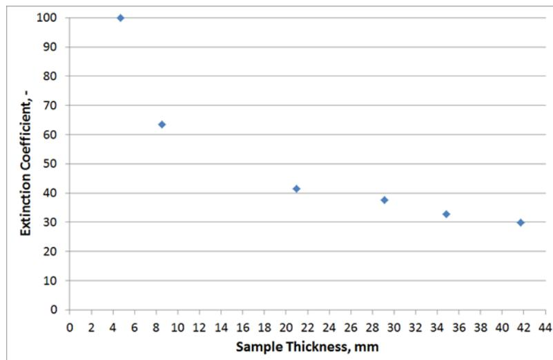
Figure 3.14. Extinction coefficient of TSA samples as function of the thickness
