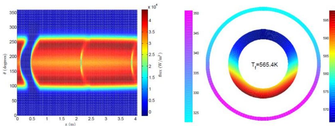
Figure 3.6 View of flux distribution on the steel absorber provided by the optical model (left) and temperature distribution at the receiver outlet section (glass envelope and steel absorber) for specific irradiation and superheated steam conditions in the receiver tube of a PTC (right).
