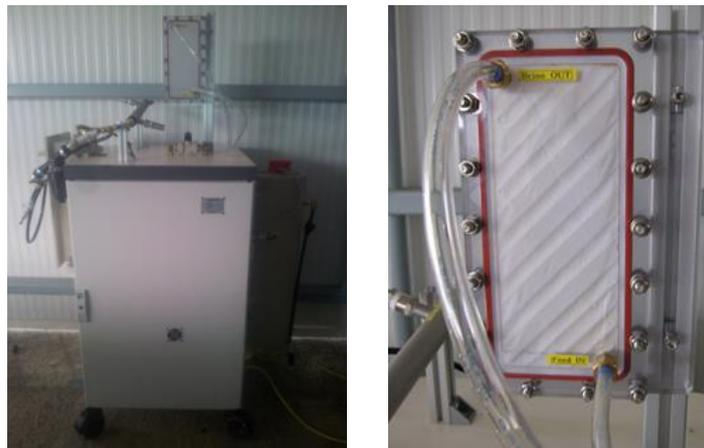
Figure 2.37. Laboratory unit for testing membranes on vacuum MD
