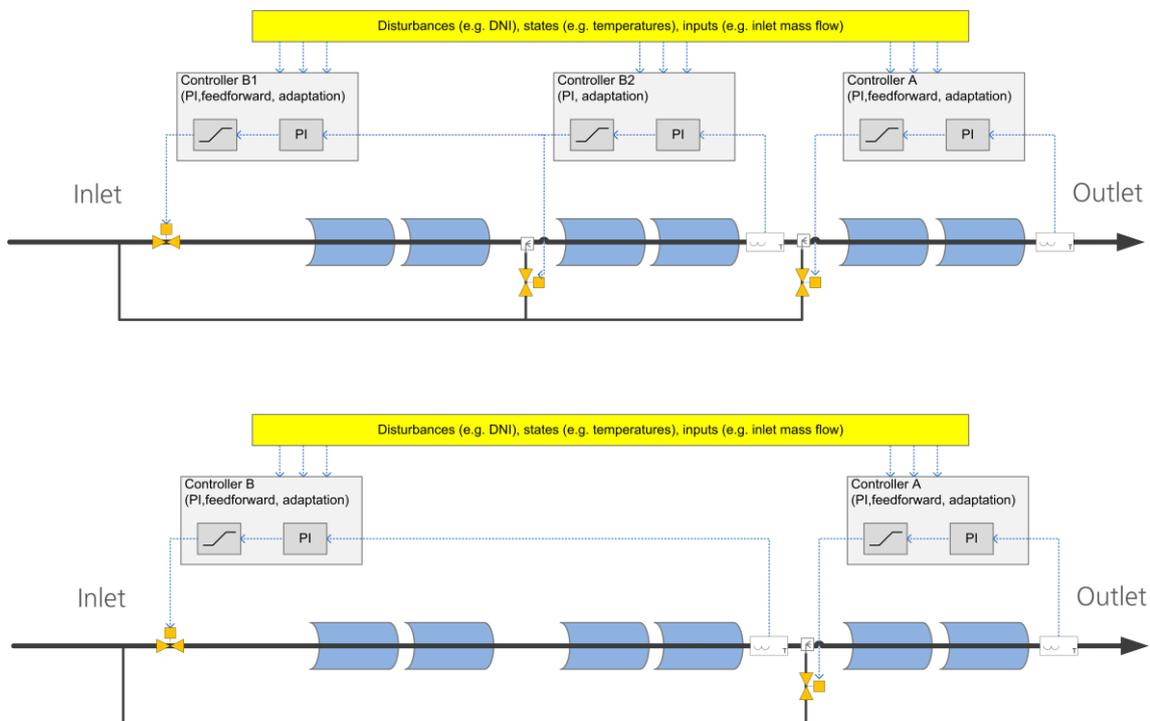
Figure 3.5. Two variants of control loop splitting (Feldhoff et al., 2014).
