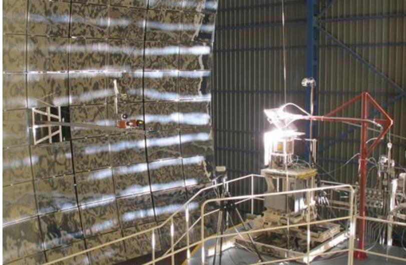
Figure 2.19. Interior view of the PSA SF-60 Solar Furnace in operation.
