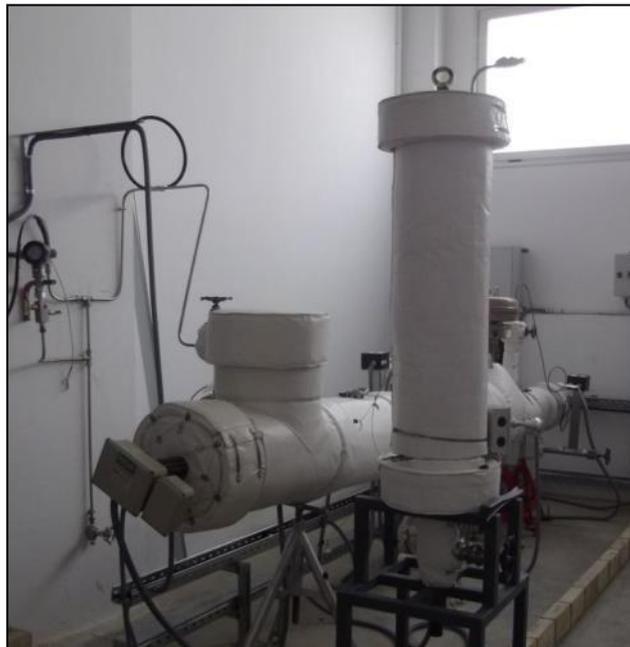
Figure 3.7. Testing device with molten salt filling oven.
