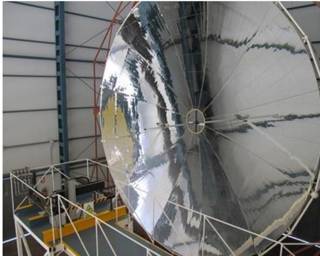
Figure 2.20. Interior of the SF-40 solar furnace, showing the parabolic concentrator.
