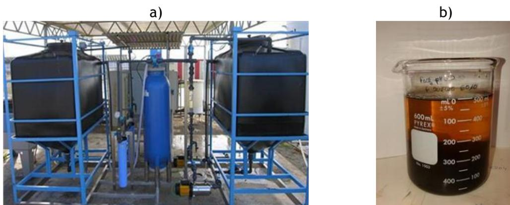
Figure 5.4. Optimization of the physic-chemical pre-treatment of cork boiling wastewater: (a) pre-treatment at pilot plant scale (500 m<sup>3</sup>/h) (b) Turbidity and total suspended solids elimination through the physic-chemical step.
